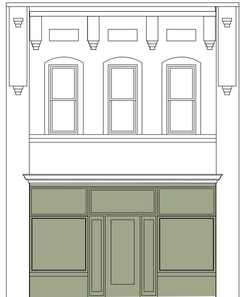
A: Remove the inappropriate storefront and rebuild the original storefront based on historical documentation. Or install a new storefront that respects the historic character of the district.
