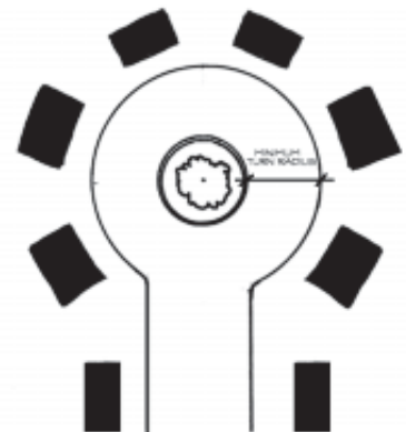
Cul-de-sacs with a minimum turn radius lessen the visual impact of asphalt in new developments.
