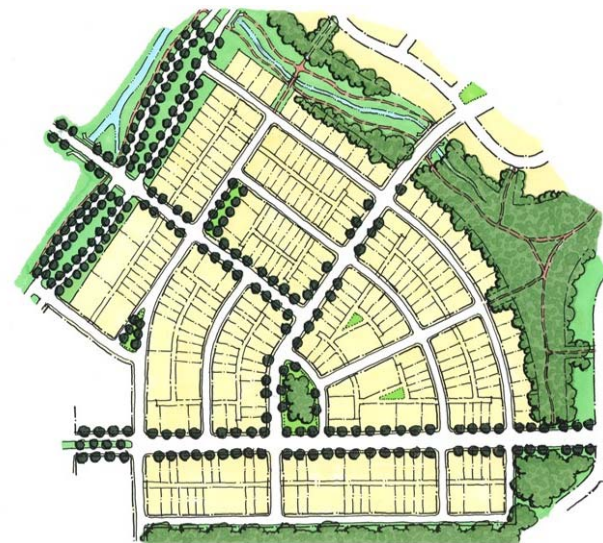
Neighborhood with Gridded Street System Courtesy Looney Ricks Kiss Architects
