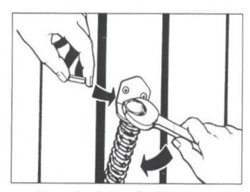
Closer springs feature adjustable torque
