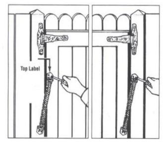
Install closer on the hinge side of the gate with the "top label" at the top as shown.
