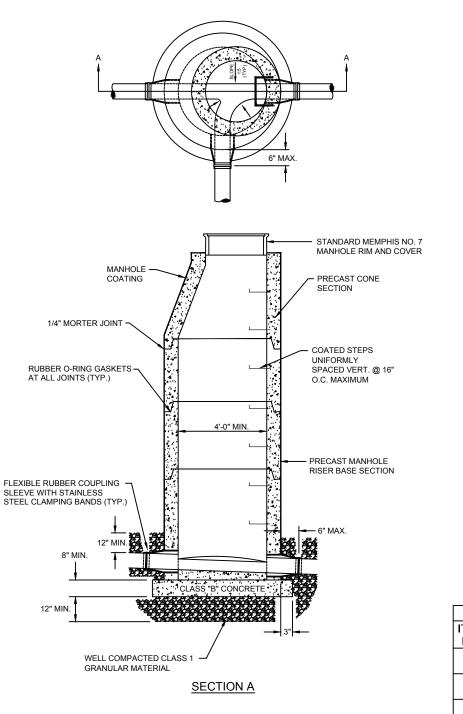
MEMPHIS NO. 7 MANHOLE RIM AND COVER, TENNESSEE NO. 3 MANHOLE CASTING WITH TYPE 'B' COVER.
