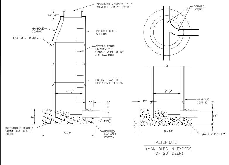
MEMPHIS NO. 7 MANHOLE RIM AND COVER, TENNESSEE NO. 3 MANHOLE CASTING WITH TYPE 'B' COVER.
