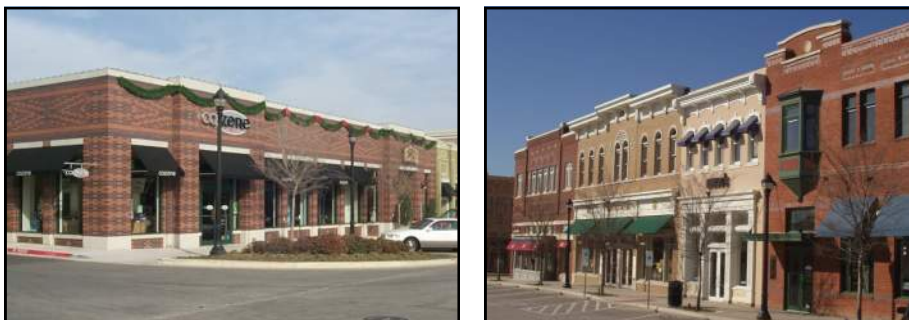
This new town center in Southlake, TX contains a mix of awning and canopies. The façade treatment including the awnings turn the corner at an intersection (above left). Awnings can be incorporated into the ground floor as well as upper floors (above
