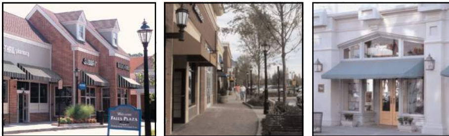
Awnings can be used to pull together a development of commercial buildings (above left) and to add color and interest and provide shade for pedestrians (above center). Awning styles can range from traditional (above right) which are often retractable to modern which are often fixed (above center).
