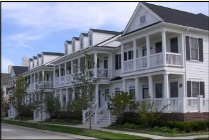
The buildings above include an articulated top, middle, and base; building length is reduced by changes in plane, roof form, porches, and details
