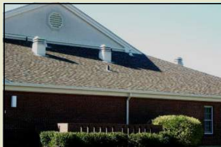
Locate roof appurtenances at back of building
