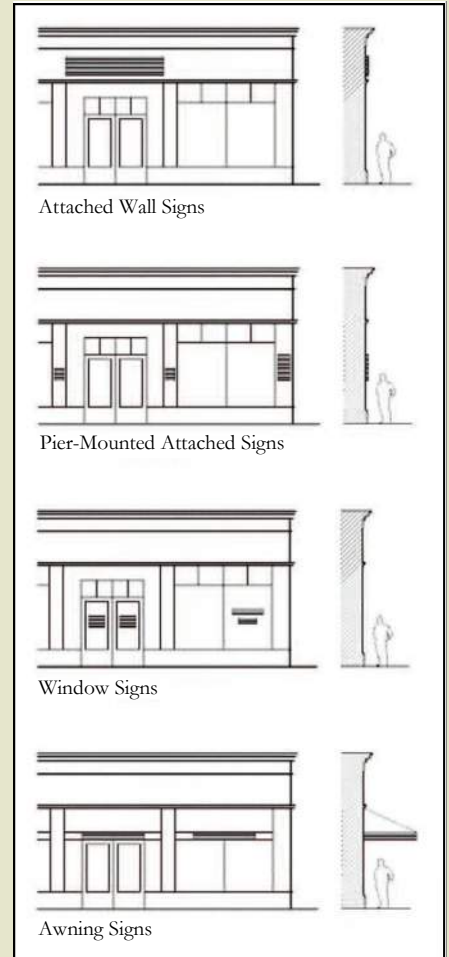
Recommended Sign Placement
