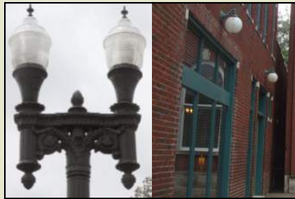
Unshielded decorative fixtures
